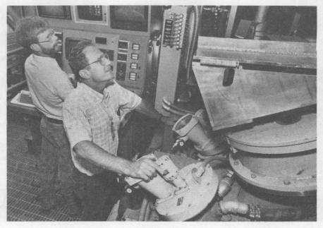
FRANK ZANNER (DMTS), and Mark Miszkiel (both 1833) operate an electronbeam furnace that will be used for some of the SMPC-related research conducted at Sandia.
